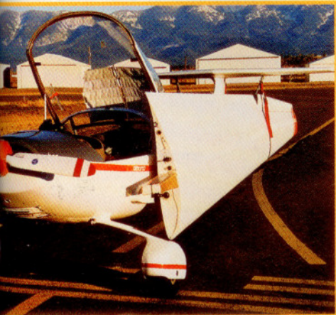
Visibility in the Dimona is excellent—its bubble canopy provides a window to the world. With its wings folded against the fuselage, the Dimona shrinks to 7 feet wide.
